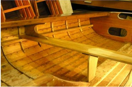
**R 154 responding to restoration with the after timbers removed and oxalic acid applied.**
